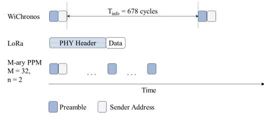
**Figure 1.** WiChronos illustration ultra narrowband (UNB) to enhance the range. The reduced time-on-air aids in system scalability.
