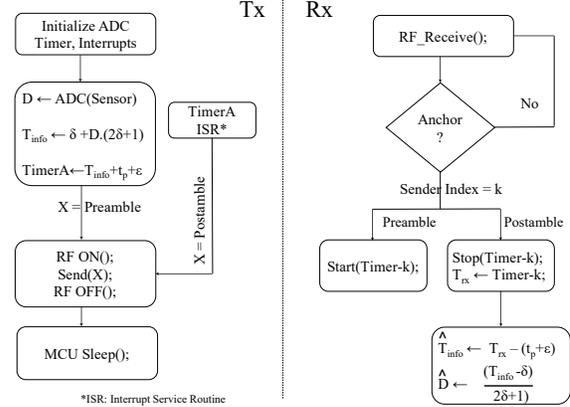
Figure 2. System implementation flow diagram
